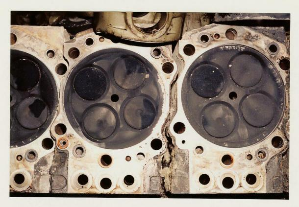
The photograph below is of the same two combustion surfaces after they were wiped with a "dry" shop cloth. As you can see there is no "hard carbon".
