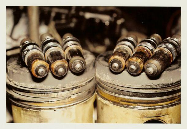
The last photograph of this series is a close-up of three of the injectors pictured above. Notice the cleanliness of the tips.
