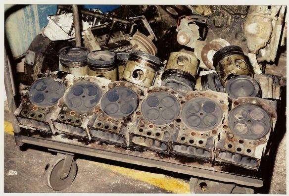
The photograph below is of the same combustion surfaces after they were wiped with a "dry" shop cloth. The result shows bare metal with no hard carbon.
